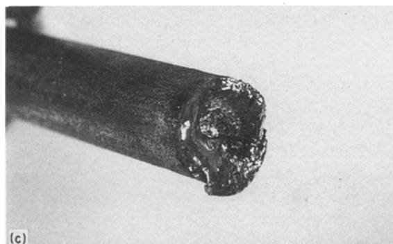
Figure 2 Internal electrode of the plasma generator (a) before the process, (b) after more than 15000 pulses, (c) free end of the electrode.
